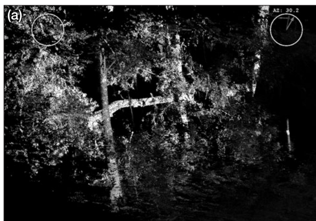
Figure 5. (a) A ground-based 3-D lidar scan taken in the forest, as shown in Figure 3b. Details such as foliage density, branch structure, stem form, and bark texture could be quantified and used for rainfall interception model parameterization. Data were collected using an Intelligent Laser Ranging and Imaging System (ILRIS) with a maximum field of view of 40° vertical by 40° horizontal. Data resolution was 9 mm, and a total of 1 251 632 laser returns were collected to generate this dataset. The 10-m wide image was created using QT Modeler software. Brightness is proportional to intensity of laser return. Circular symbols refer to the reference ILRIS instrument elevation. EL = meters from the ellipsoidal height and AZ = azimuth in degrees from true north. (b) A 3-D ground-based scan of a longleaf pine sandhill ecosystem at the Ordway-Swisher Biological Station near Melrose, FL ( www.ordway.ufl.edu ). The 7-m x 5-m image was generated using ILRIS data collected at a 1-cm point spacing and field of view of 40° vertical by 40° horizontal. The colors represent height gradients, with blue corresponding to the ground surface and red corresponding to the upper canopies of the tallest trees.
